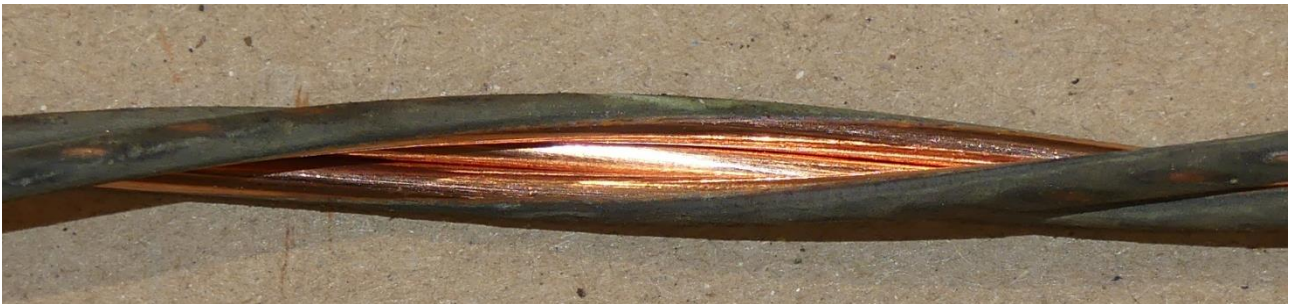
Figure 7 Inner surface of inner copper strands – Tag ID 140
