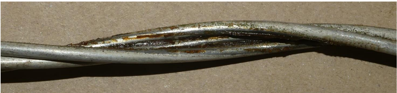
Figure 2 Inner surface of outer aluminium strands – Tag ID 271
