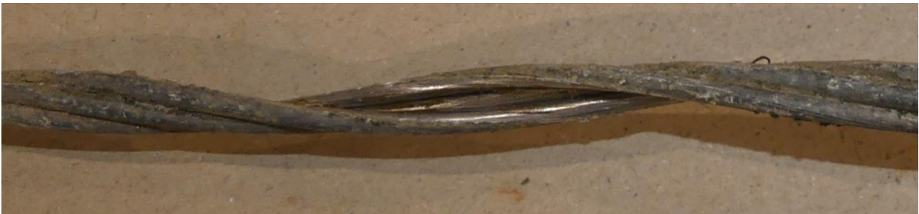
Figure 10 Inner surface of outer aluminium strands – Tag ID 005
