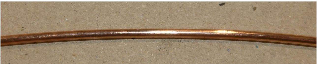
Figure 8 Condition of core copper strand – Tag ID 140
