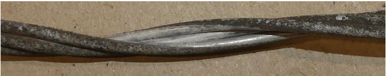
Figure 13 Inner surface of outer aluminium alloy strands – Tag ID 001
