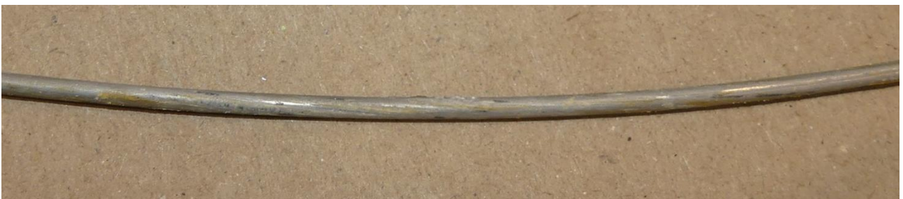
Figure 14 Condition of core aluminium alloy strand – Tag ID 001
