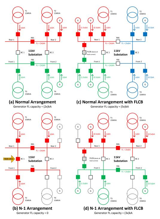
Figure 8 - Operating scenarios for a 4x15MVA substation, with/without a FLCB
