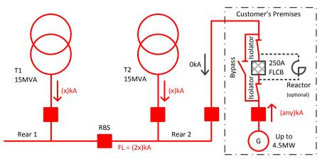
Figure 18 - Schematic diagram of Method 2 trial
