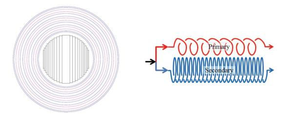
Figure 15: Mutual reactor winding scheme: use of standard transformer design specifications and materials produce a robust, high efficiency module
