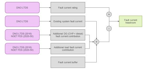
Figure 3 Schematic representation of data sources used to calculate fault current headroom
