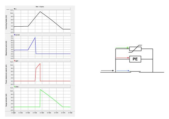
Figure 5 - Line current and currents through the mechanical switch and the power electronic switch and the surge arrester.
