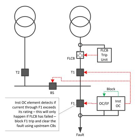
Figure 11 - Independent backup protection option 2 – CB Fail Approach
