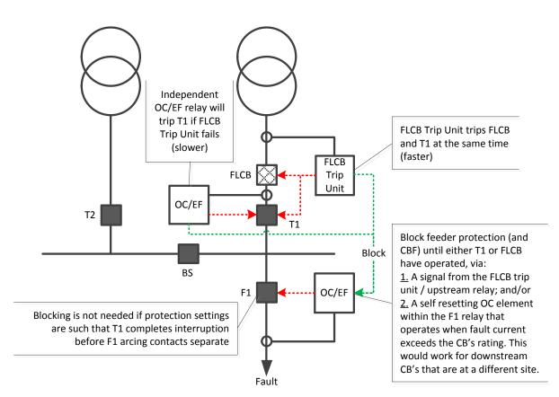
Figure 10 - Independent backup protection option 1 - Adaptive Protection
