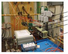
Surge arresters IGBT switches Mechanical switch Electronic and actuator energy for the mechanical switch Fault current limiter logics control the mechanical and the power electronic switches
