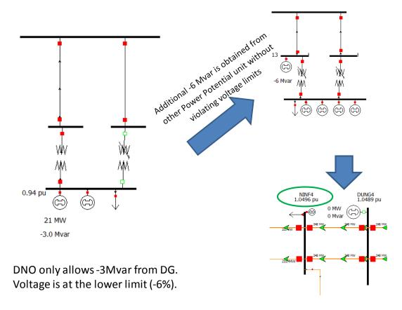
Figure 8 A solution from the Power Potential approach
