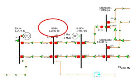
Figure 5 An overvoltage problem at the transmission
