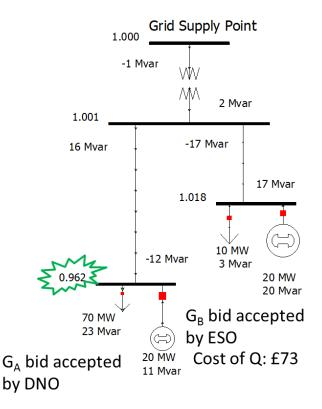
Figure 12 ESO-DSO's no coordinated solution
