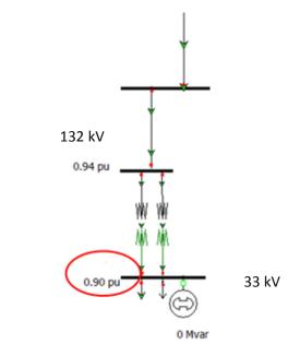
Figure 26 Undervoltage problem in Power Potential distribution grid
