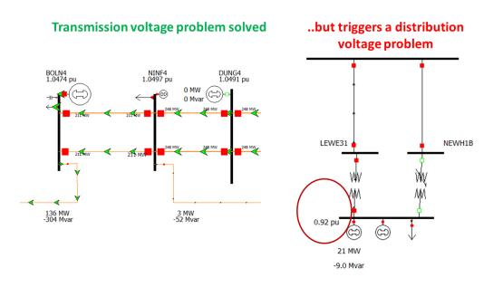
Figure 7 An undervoltage problem caused by non-coordinated DSO-ESO control actions
