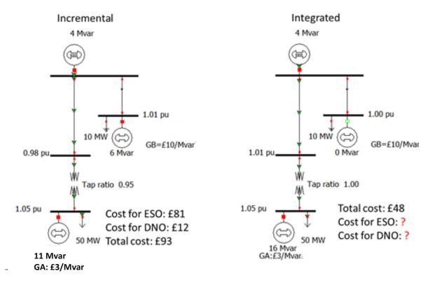
Figure 24 Comparison between the incremental and integrated solution with no smart (preventive) control
