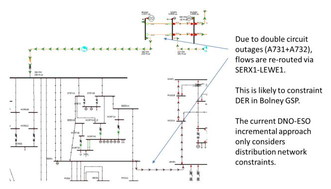
Figure 31 Impact of transmission outages on the distribution system
