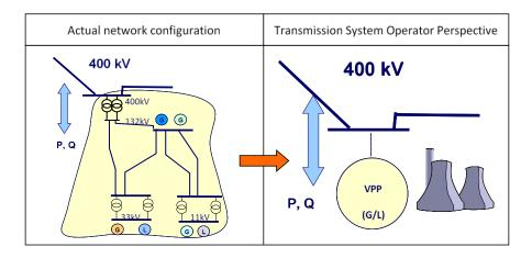
Figure 1 Characterisation of DER as a Virtual Power Plant
