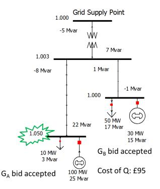
Figure 4 A solution from the Power Potential approach
