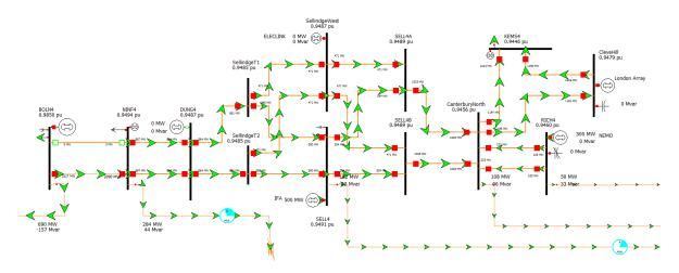
Figure 37 A system with high demand (winter), low import, and a 400 kV circuit outage between Bolney and Ninfield
