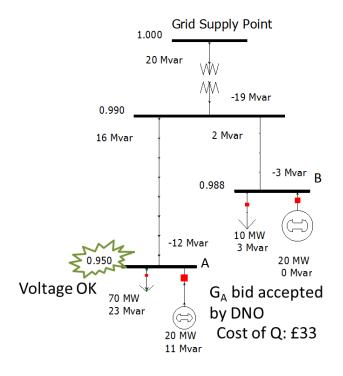
Figure 13 Step 1 of DSO-ESO incremental approach: DSO solution for the undervoltage problem at the distribution
