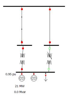
Figure 6 A transformer circuit outage in Ninfield distribution area
