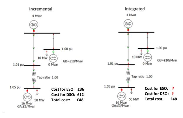
Figure 25 Comparison between the incremental and integrated solution with smart (corrective) control
