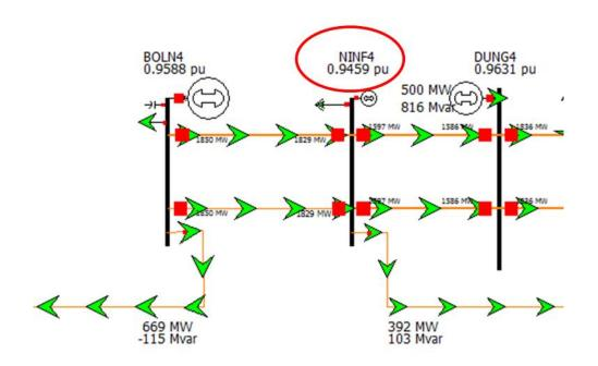
Figure 27 Undervoltage problem at the transmission
