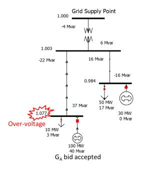
Figure 3 An overvoltage problem caused by no ESO-DSO coordination
