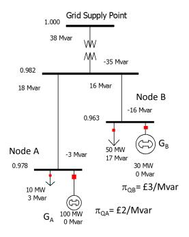
Figure 2 A distribution system with DER
