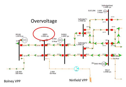
Figure 16 Overvoltage at Ninfield 400kV
