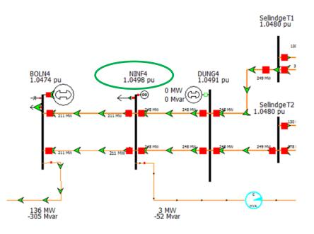
Figure 18 A power Potential unit in Ninfield VPP is used to correct the overvoltage problem at Ninfield 400 kV
