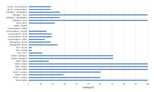
Figure 4-4 Loading of each circuit after redispatching the output of VPP and transmission connected generators
