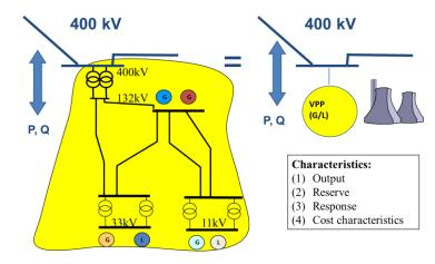
Figure E. 6 VPP as a flexible representation of the aggregated DER and networks
