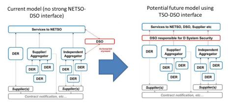
Figure 2-2 A potential future model of TSO-DSO interface<sup>6</sup>
