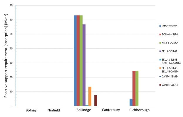
Figure 5-2 Reactive power requirement in different system conditions
