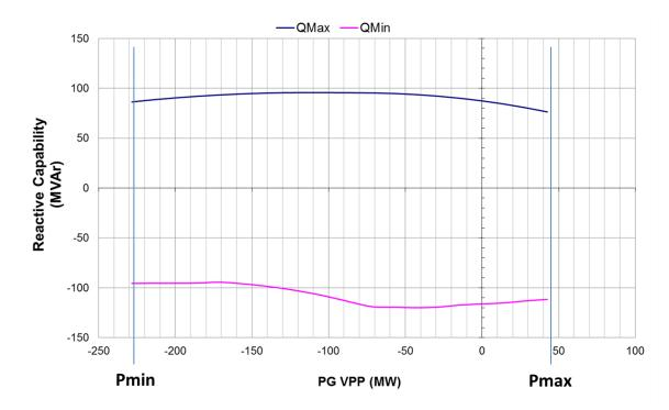
Figure 3-12 PQ curve of the Canterbury VPP
