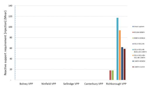
Figure E. 3 Optimal volume of reactive power injection needed from each VPPs
