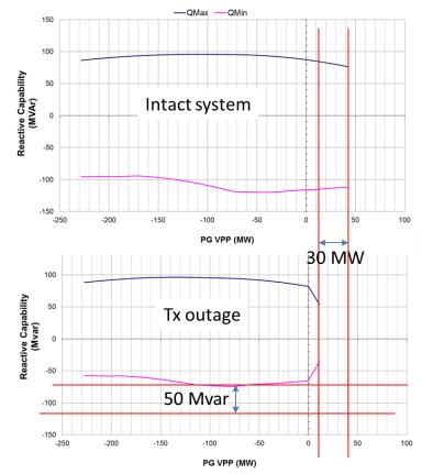
Figure E. 11 Impact of a transformer outage on the PQ curve capability of Canterbury VPP
