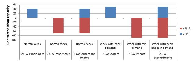
Figure 2-17 Allocation of reactive power contract to VPP A and VPP B depending on the system conditions forecasted a week ahead
