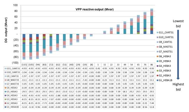
Figure 3-22 Reactive power dispatch of each DER in Canterbury VPP
