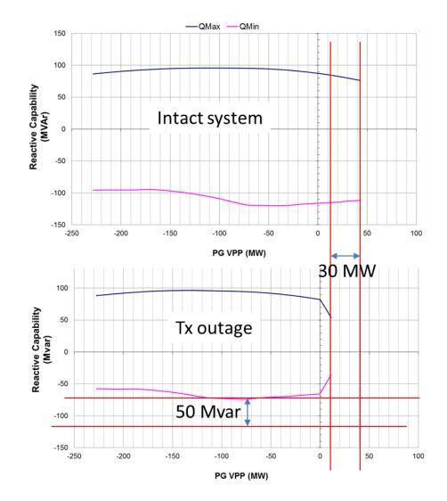
Figure 3-20 Impact of a transformer outage on the PQ curve capability of Canterbury VPP
