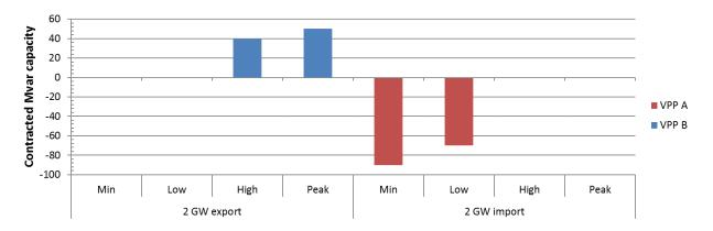
Figure 2-16 Allocation of reactive power contract to VPP A and VPP B depending on the system conditions forecasted a day ahead
