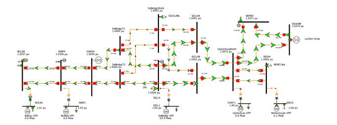
Figure 4-6 Solving network over-voltage problem using VPP
