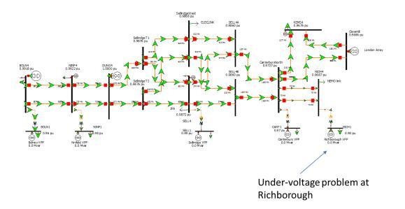
Figure E. 2 Illustration of the under-voltage problem that can be solved using DER services
