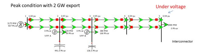
Figure 2-6 An illustrative example showing an under voltage problem during peak load condition with 2 GW export
