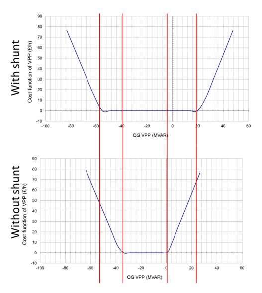
Figure 3-18 Mvar cost function [Sellindge VPP] with and without shunt reactive compensator
