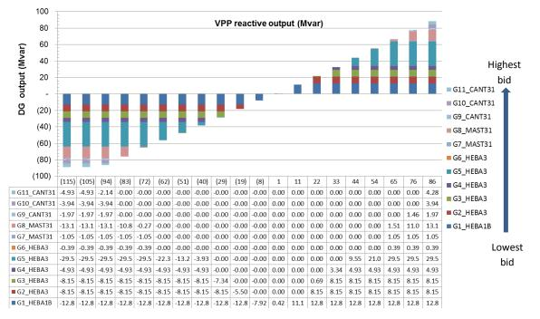
Figure 3-21 Reactive power dispatch of each DER in Canterbury VPP
