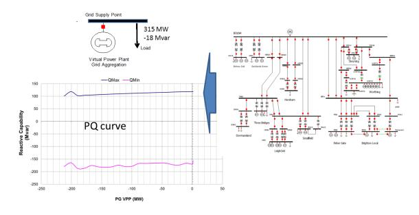
Figure E. 7 Reactive power capability and its cost function of Bolney VPP
