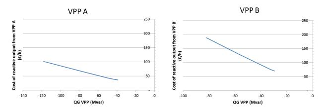
be £78/h. If VPP B is selected, then the cost of contracting 50 Mvar (lag) from VPP B is £90/h. Therefore, the solution is to contract VPP A resulting in lower cost.
