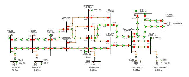
Figure 4-1 South-East GB transmission test system
