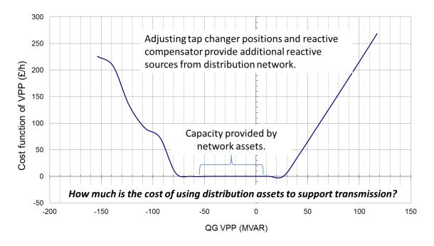
Figure 3-17 Mvar cost function [Bolney VPP] with optimised tap changers and distribution reactive assets
