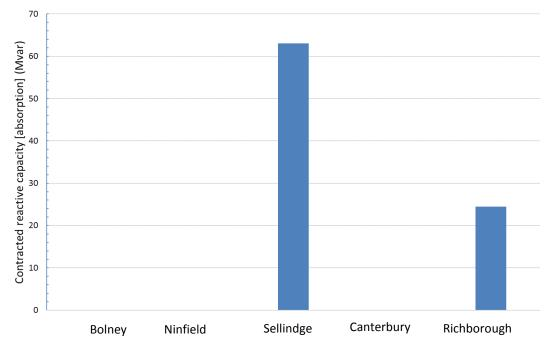
Figure 5-3 Contracted reactive capacity for the summer peak condition
