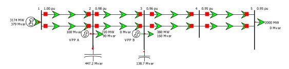
Figure 2-10 Solving the under-voltage problem using 100 Mvar from VPP A
