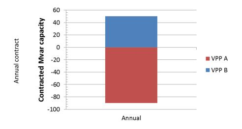
Figure 2-18 Allocation of reactive power contract to VPP A and VPP B depending on the system conditions forecasted a week ahead
