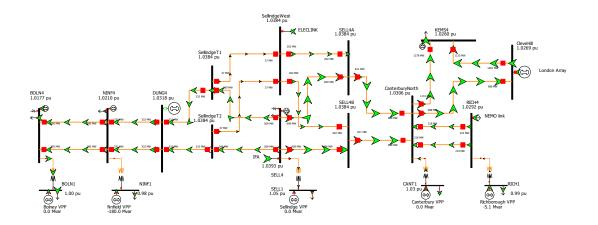
Figure 4-8 Solving network congestion problem using a combination of the transmission connected generators and VPPs
