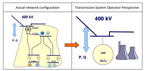
Figure 2-4 Characterisation of DER as a Virtual Power Plant
