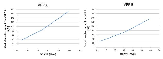
Figure 2-14 Cost function of reactive power services (injection) from VPP A and VPP B during peak demand<sup>7</sup>
