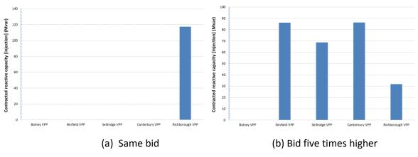
Figure E. 4 Optimal volume of reactive power contracts allocated to different VPPs for different bids
