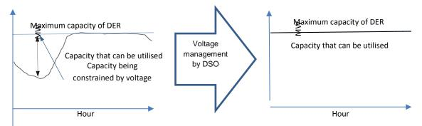
Figure 1-1. An illustrative example of the increased role of DSO to enable full access to DER capacity to provide transmission services
