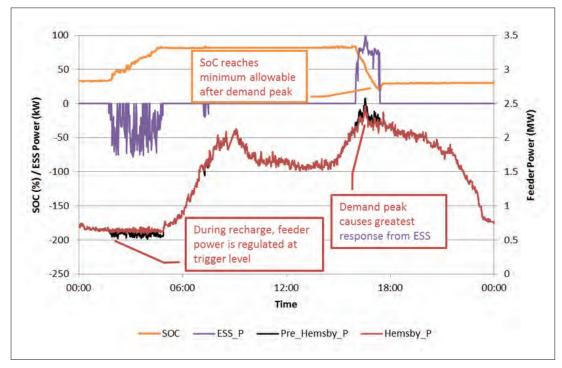
Figure 1 - Results from one day of peak shaving (load shifting)
