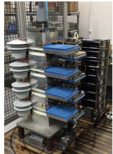
Figure 17: First test assembly of the FLCB
