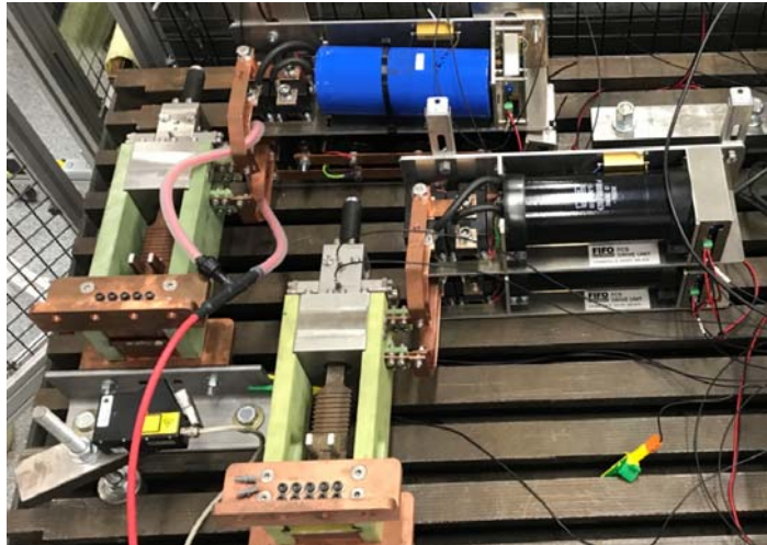
Figure 43 – Mechanical endurance test set-up
