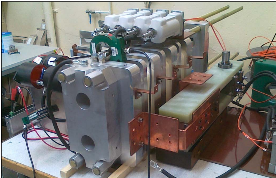
Figure 9 – FLCB single-phase proof-of-concept prototype (TRL4) from ABB's R&D project that the Powerful-CB project has developed further)
