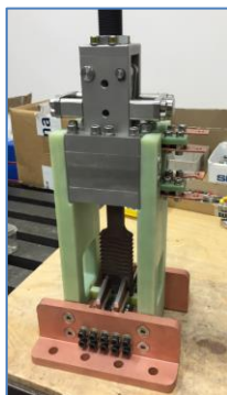
Figure 4. One of the Fast Commutation Switches used for the Powerful CB.
