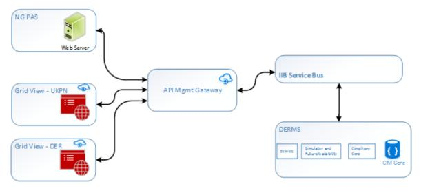
Figure 12: the Azure APIM Gateway and IIB architecture
