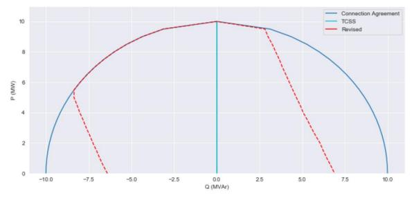
Figure 21: An example PQ capability curve
