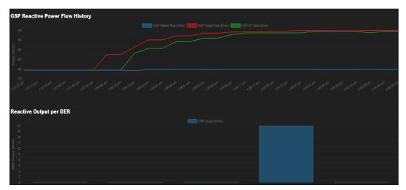
Figure 16: Example of stable testing result. One DER available: Q actual tracks (green) Q requested (red) for the following instruction: voltage set point of 405kV, dead-band = 2kV, 4% drop.
