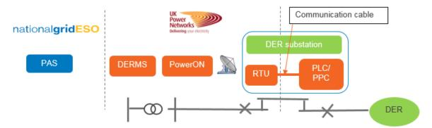
Figure 34: Communications link focussing on DER substation
