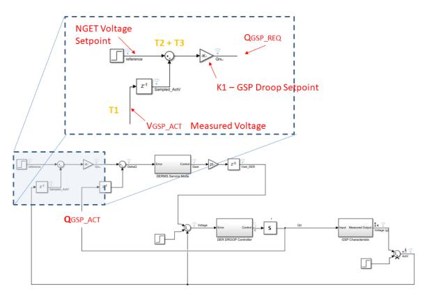
Figure 14: DERMS Q service mode control system (view 1/2).
